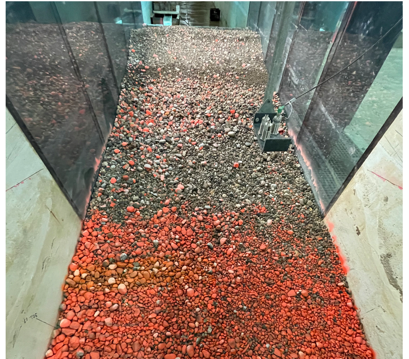
After testing. Waves have moved and mixed cobble.
